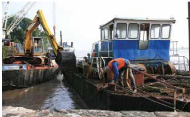
. . . Fred's dredger Riparian being used to manoeuvre the old vessel, often using the bucket of the digger on board.
