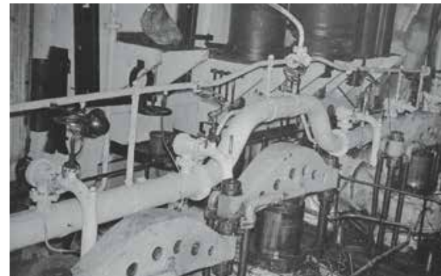
The top exhaust pistons.
