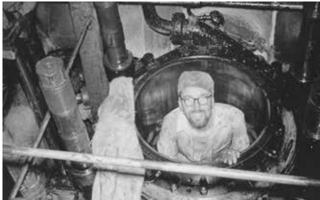
All pictures are of a B&W engine. Roger Inglis is in the cylinder, having just de-coked the top exhaust ports.
