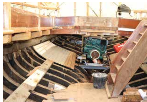
A general view of the deck of Britannia, showing the large cabin space that was added when owned by a training organisation. The plan is to return this area back to its much smaller original size.
