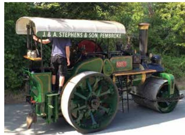
Robey three-point roller, built 1913, No.32387, which resides in the collection in complete, running order.
