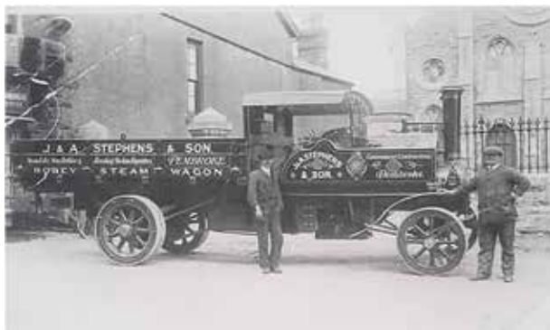
An early 1906 Robey overtype lorry, also once part of the J & A Stephens fleet in Pembrokeshire.
