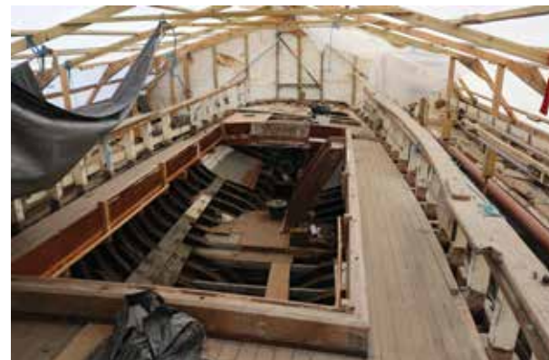
A general view of the deck of Britannia, showing the large cabin space that was added when owned by a training organisation. The plan is to return this area back to its much smaller original size.
