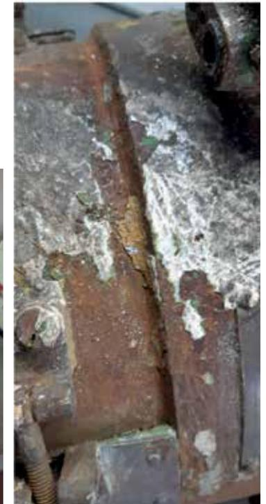
were peeling away and the underlying casting was quite corroded. Fortunately before the lockdown came into place, the motor and fan had been disconnected from the ducting and the cabling, so lent itself to being temporarily removed from the ship to be worked on.
