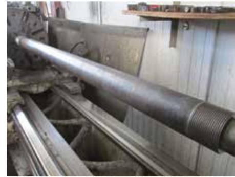
*The long bed lathe for screw cutting the consecutive thread with a single point tool.*
