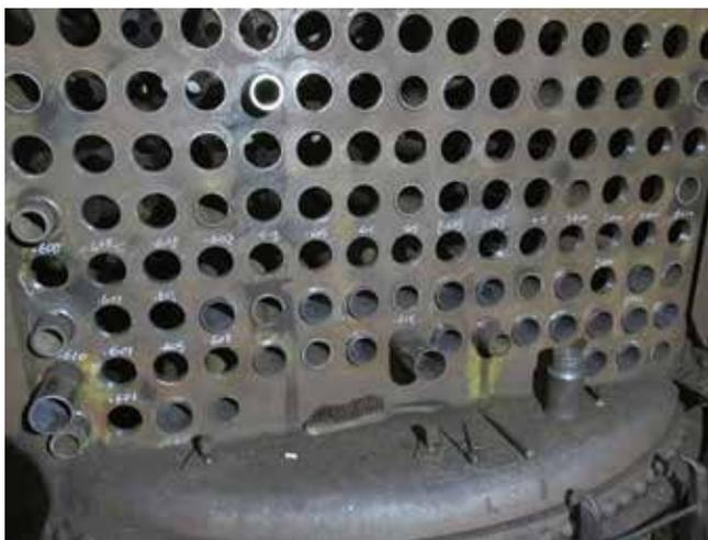
*View of the smokebox end showing the variation in tube hole diameters from 2.600ins upwards. The five stay tubes with their tack welded sockets are in position. Access and space at the firebox end of the boiler is limited as the bulkhead here is close to the boiler. Precious little room for two men and the air tool expander, hose, and various tooling.*
