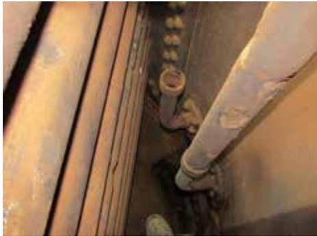
*The holed feed pipe, and the second pipe missing.*
