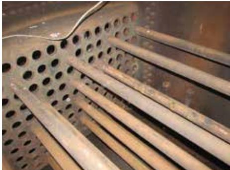
*The stay tubes after removal of the flues. The third tube on the right (D5) can be seen badly pitted.*
