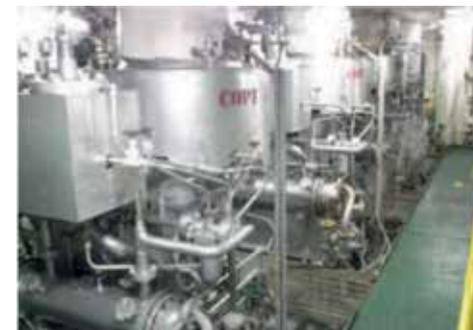
directing them to the turbine blades forcing them to rotate the shaft. The rotational power generated is then transmitted to the centrifugal pump through a connected shaft. Any excess steam travels through the exhaust to a vacuum condenser where it condensed back into water and then goes back to the boiler via a feed water pump.
