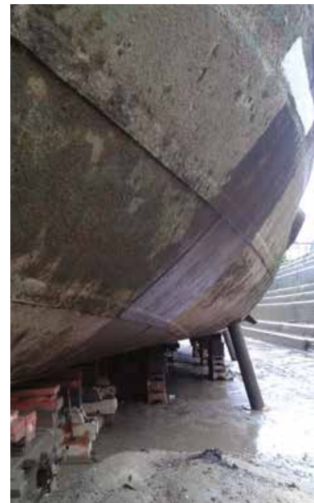
The hull plates can now be seen as they await cleaning.
