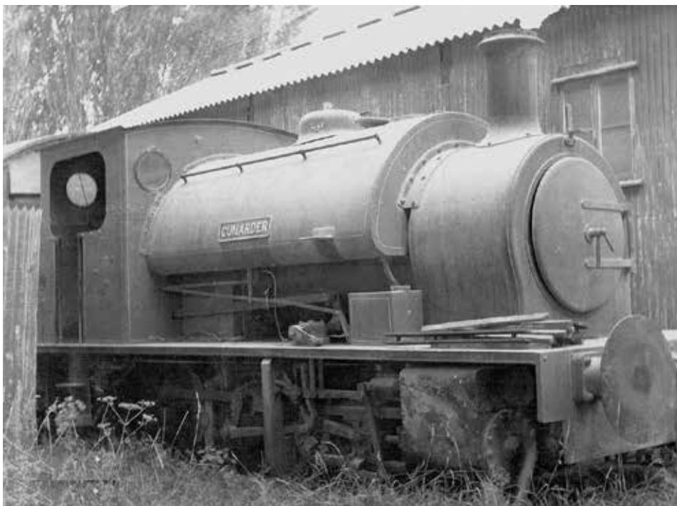
Cunarder as purchased in 1969 from store at Blue Circle Cement Works at Harbury in Warwickshire. Note the large short reach buffers fitted to work short radius curves without locking buffers.
