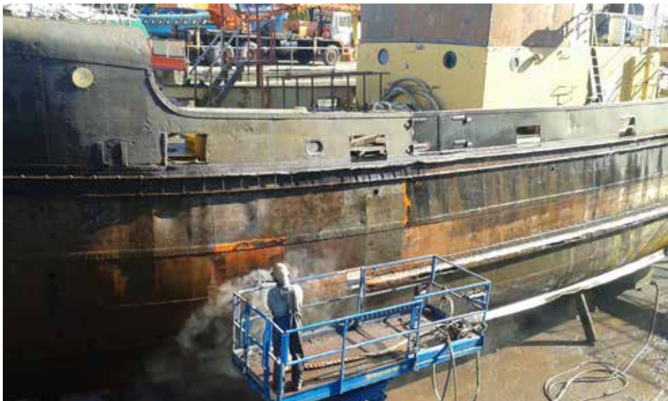
Water blasting is well underway in this view of Freshspring.
