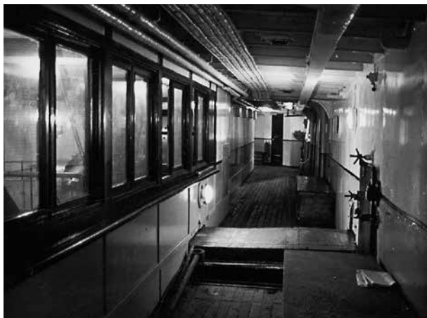
Looking down the passageway alongside the engine room with the step over the paddle shaft visible.
