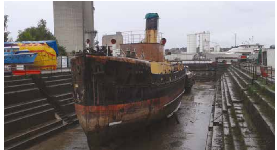
The dock has been pumped out and Freshspring sits on the blocks.
