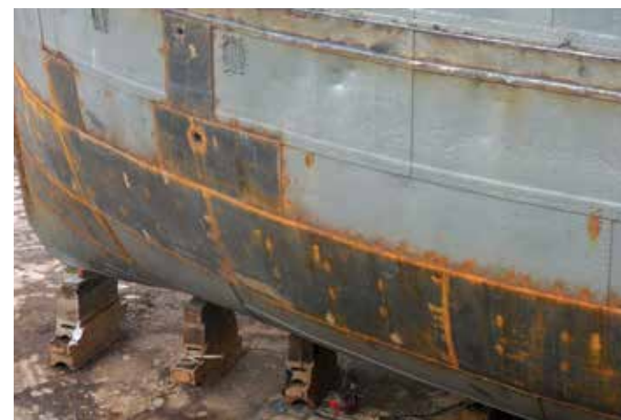
The port side bow area needed a fair bit of plating.
