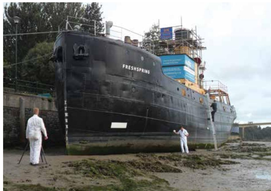
The team from BMT Defence Systems at work mapping the ship's hull.
