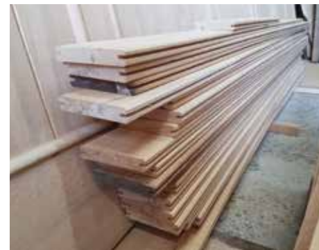
Machined tongue and groove for the panelling ready for the remaining two sides of the wheelhouse.
