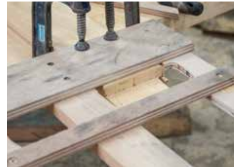
Jig for cutting the tenons to aid accuracy and efficiency.
