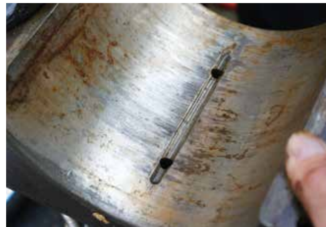
Top half of rear bearing upside down – the grey colour shows the heavy pressure areas.
