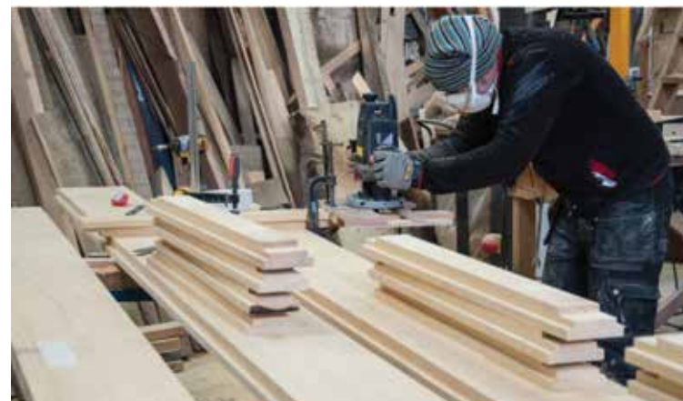
Keith cutting the tenons on the ends of the stiles. The three rails for the front panel can be seen underneath.
