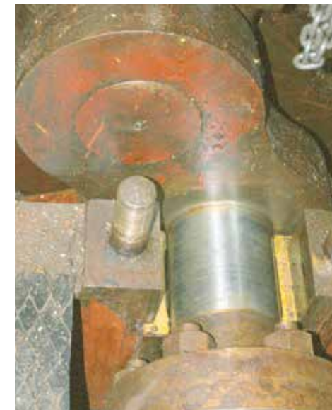
The main bearing at the rear of crankshaft – the journal is in good condition.
