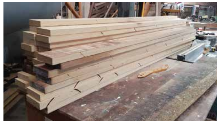
Machining up the Iroko for the panelling from rough sawn boards.
