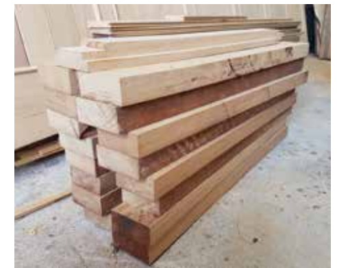
Stiles for the two wheelhouse sides ready for machining.
