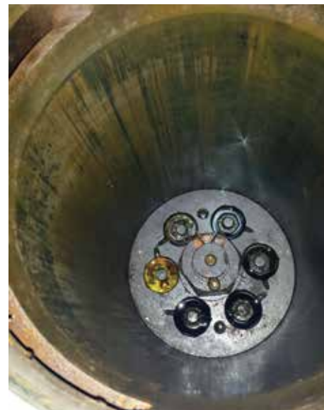
HP cylinder bore showing the top of the piston. Photo D Jackson
