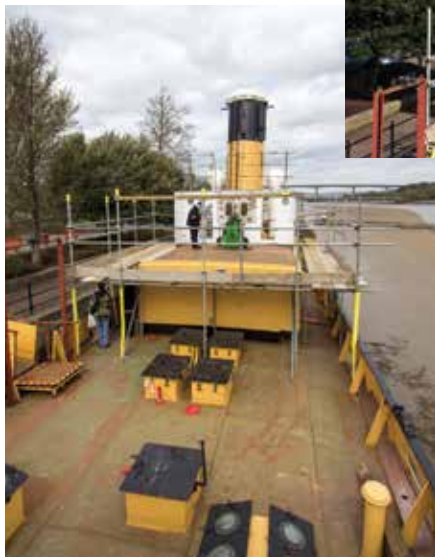
With the old plywood removed, the next step was to prepare the base for the new wheelhouse.
