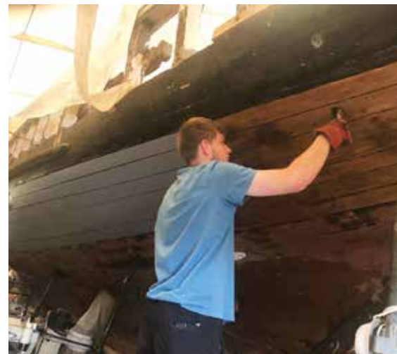
Seb applies paint to the new hull planks.
