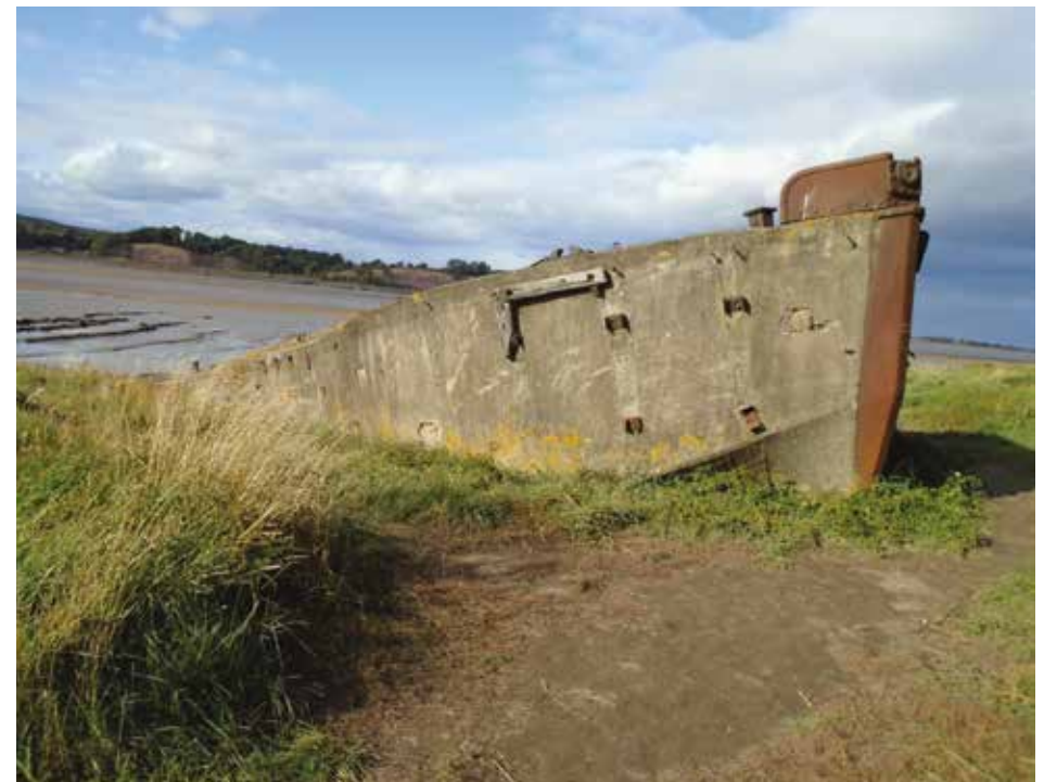
One of the concrete barges beached at Purton to shore up the bank of the canal.
