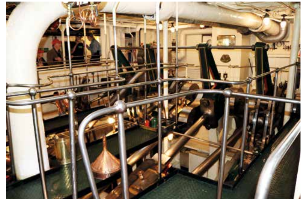
The crankshaft end of Waverley's engine. Note the shiny oil cans and brass funnel.
