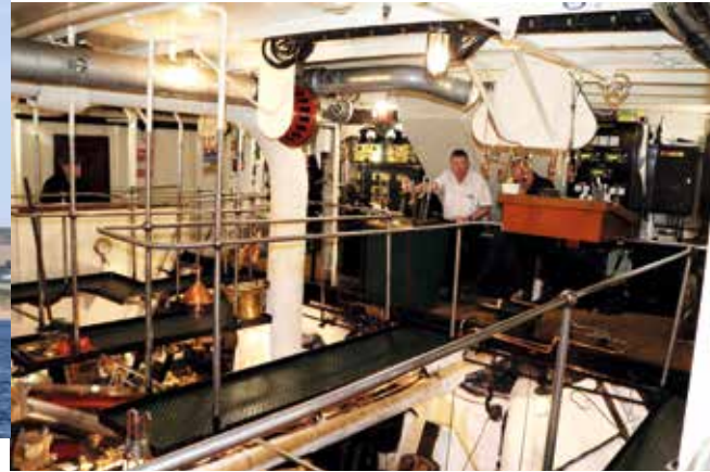
The engine of the Waverley is on full view. This shows the Engineer's driving position.
