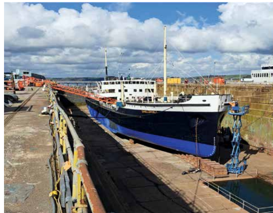
In No.4 drydock at Falmouth for annual docking and survey, April 2023. Blue antifouling applied in 2022 is a biocide free coating with Silicon to reduce marine growth.
