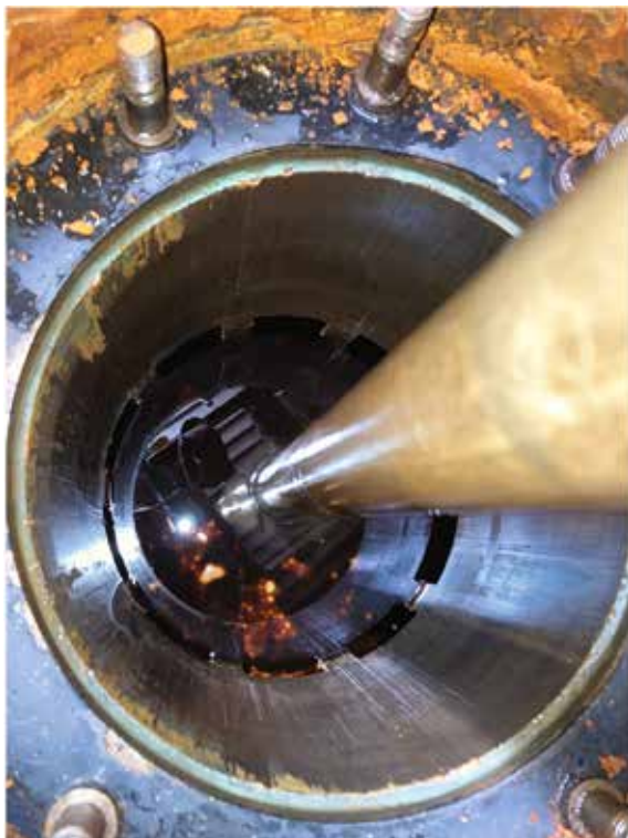
Here is a view looking into the cylinder with the piston still in place where you can see the inlet ports at the bottom. The cylinder walls are lovely and shiny.
