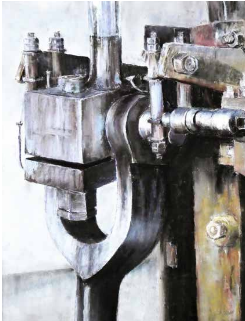
This detailed pastel painting by Rob Reed focuses on an essential part of any steam engine. The crosshead joint, which is shown, eliminates sideways forces on the piston caused by the rotation of the crank. Forces are taken by the crosshead guide or slide, which can be seen behind the joint. The engine on SS Freshspring is inverted, which means the cylinders are above the crankshaft and so, in the painting the piston rod is at the top and the connecting rod is shown below. From the painting we can even determine that this is the high pressure piston, which has the rocking lever drive to the air pump as described by Richard Slack in his excellent article.
