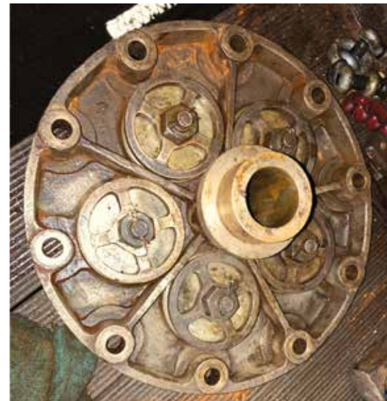
Valve plate after cleaning (lovely machined brass plate and valves).
