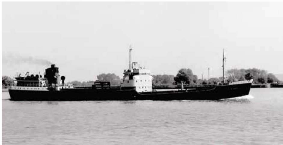
SS Cliffe Quay, built 1950, was the last coal-fired steam collier owned by the Central Electricity Generating Board. Seen near Beckton in July 1977. Reg Batten
