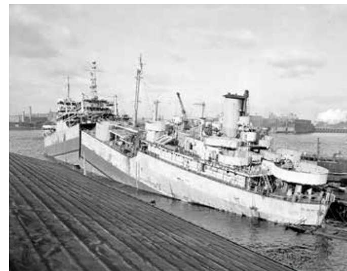
The Ponanganset which split in two while in harbour.
