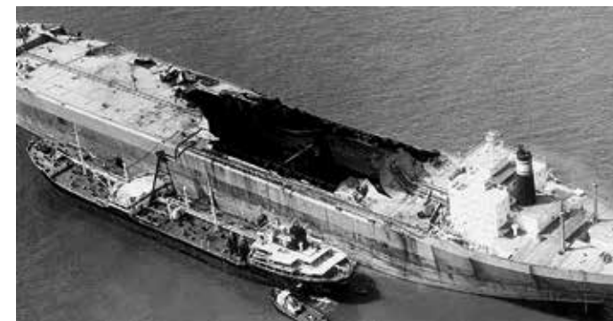
Kong Haakon VII after an explosion which ripped a 100 metre hole in her deck.
