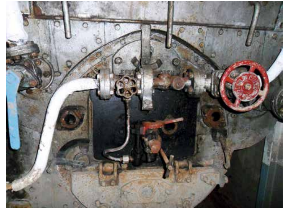
Starboard oil-fired furnace on SS Freshspring .
